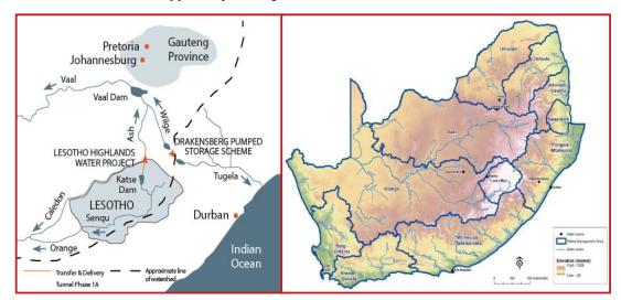
The Tugela-Vaal Transfer Scheme and Lesotho Highlands Water Project (Fig. 9 left) supply water to the Vaal catchment (Fig. 9 right). The Drakensburg Pumped Storage Scheme, completed in 1981, also contributes electricity to the national grid through hydroelectric generation as water passes through turbines at four dams down the escarpment. Most significantly, water is imported from Lesotho after being collected in the Katse Dam, and piped through to Johannesburg and the entire Vaal catchment.
